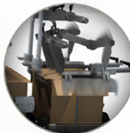
Timing and motion of case squaring and compression for sealing the case
