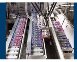
**Presto Dual Collation Top Loader** Collating and placing your products into cartons, cases or trays from two incoming lanes with the speed and precision of a Delta Robot
