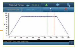
Internal oscilloscope, to view weighing/dynamic test and vibration screen
