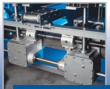
Gears are enclosed in a lubricating oil bath to eliminate wear from friction and increase machine life.
