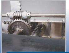
Spring-loaded compression rollers compensate for varying case heights and ensure a secure seal.
