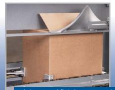
Chain-mounted flight lugs square each case during transfer.
