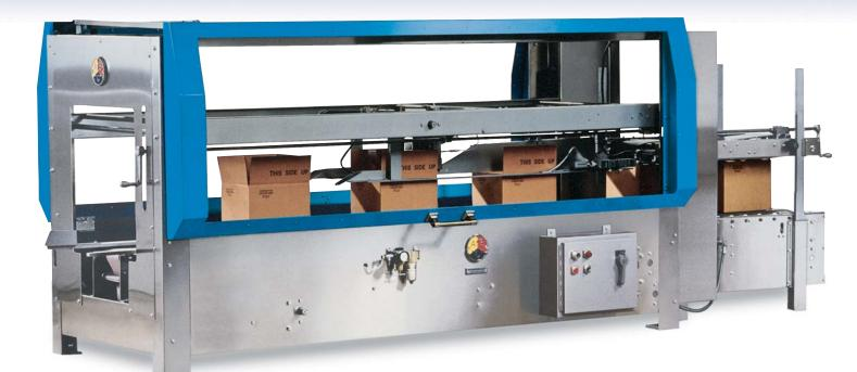
From infeed to exit, this sealer is completely automatic and needs no operator.
