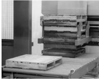
Multi-size pallet dispenser with roller conveyor
