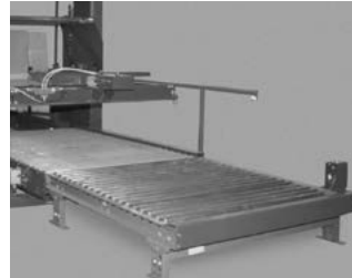
5' gravity discharge roller conveyor
