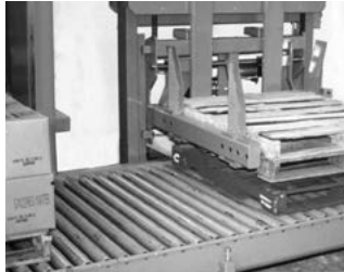
Roller conveyor for full or empty pallets
