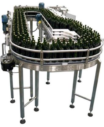
Garvey Corporation has been a forerunner in creating accumulation solutions for the wine industry. With reverse tapered bottles, expensive product and delicate labels, the wine industry needed a way to multi-lane or single-file and accumulate at high speeds, but with no back pressure. The Infinity is the Answer!
